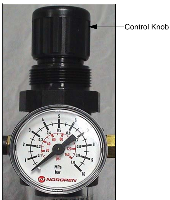
Figure 4-4: Air Regulator for Videojet 2340, 2350, and 2360
