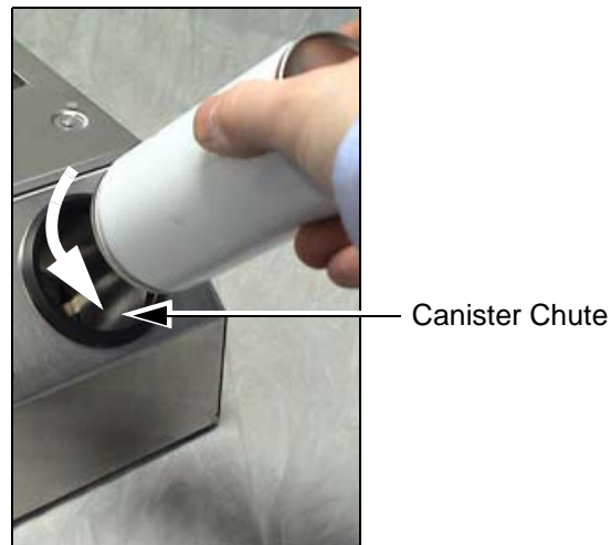
Figure 4-12: Removal of Empty Ink Canister
