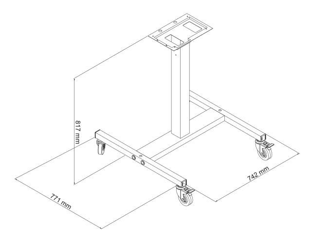
Figure A-3: Mobile Printer Stand Dimensions
