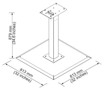
Figure A-4: Static Printer Stand
