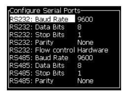
Figure 4-21: Configure Serial Ports Dialog Box
