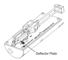
Figure 6-7: Clean the Deflector Plate (Videojet 1620 UHS - 50 Micron)
