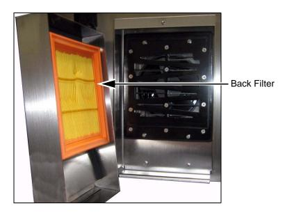
Figure 3-10: Back Filter (IP65 Version)
