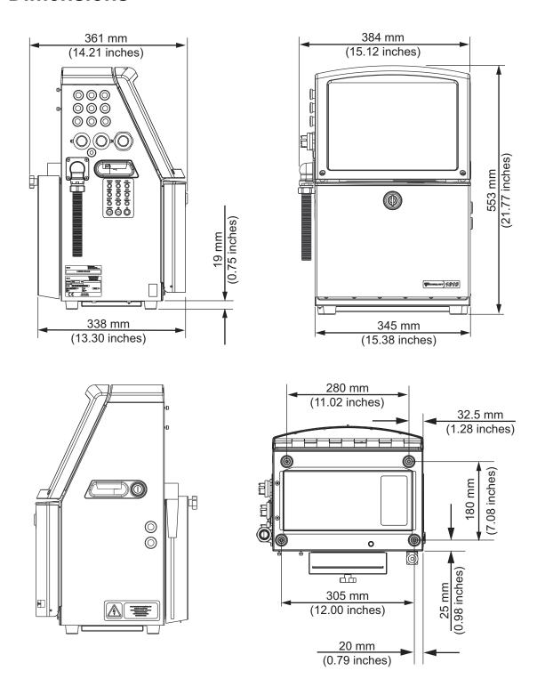
Figure A-1: Printer Dimensions
