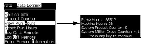
Figure 4-18: View Machine Run Hours
