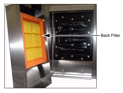
Figure 3-11: Back Filter (IP65 Version) - Videojet 1520
