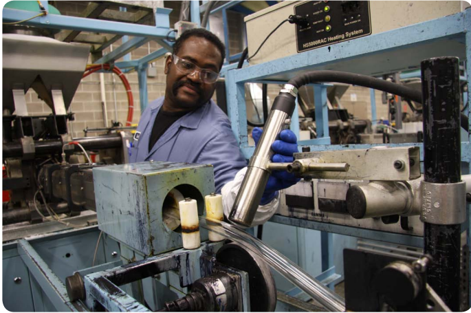
Uponor operator Mark Morgan adjusts the printhead on the Videojet 1620 continuous ink jet printer
