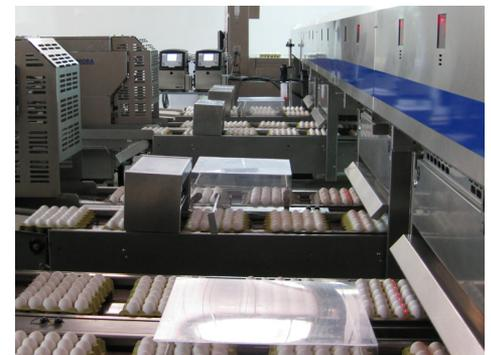
CIJ printers installed on grader
