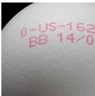
CIJ deposits ink on the surface of the egg and poses little risk to the integrity of the egg's surface because the drying process bonds the ink to the shell.
