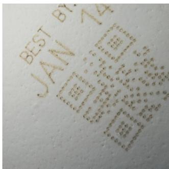
Laser marking is a process of ablation, where the laser etches the top surface of the egg. It 'bleaches' the surface of brown eggs and darkens the surface of white eggs.
