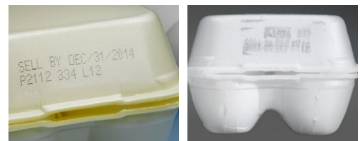
Inkjet on polystyrene carton Poor stamp code on carton
