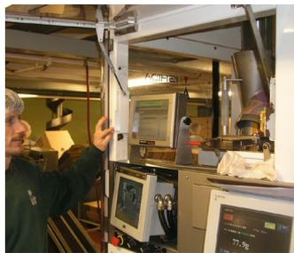
Thermal transfer overprinters feature a printhead and ribbon that make contact with a flexible substrate and create real-time images, including clean, high-resolution bar codes, text and graphics. For Utz, any product coding machine has to be robust enough to handle high line speeds while producing consistently readable codes. That was not the case with Utz's hot stampers, and also one of the reasons Epley first brought in thermal transfer printers.
