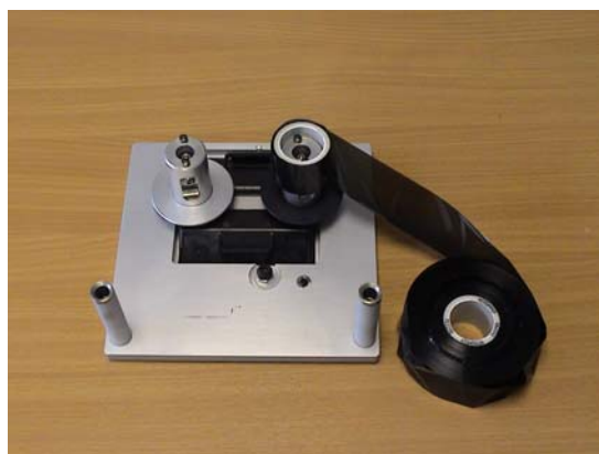
Figure 5-11: Ribbon Spools Removal
