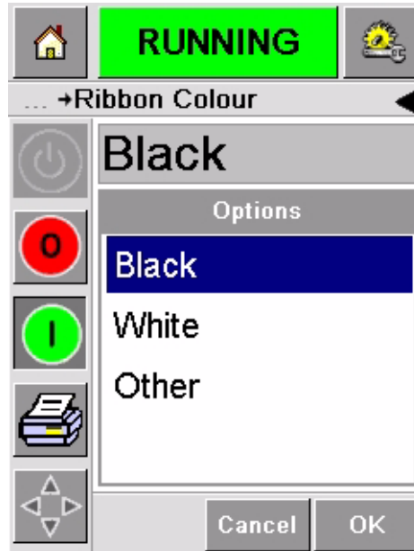
Figure 5-15: Ribbon Color Setting
