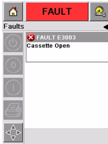
Figure 5-5: Cassette Open Fault
