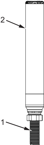
Figure 3-9: Printhead and Umbilical (Videojet 1520)
